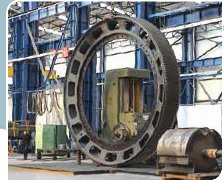
RIM GEAR FOR CEMENT MILL Ø : 5400 m : 30 (Set Group- Ankara Plant)
