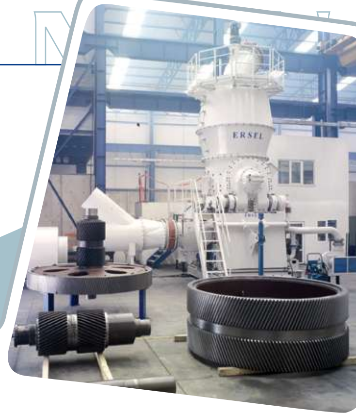
VERTICAL MILL AND GEARS FOR CEMENT MILL GEARBOX
